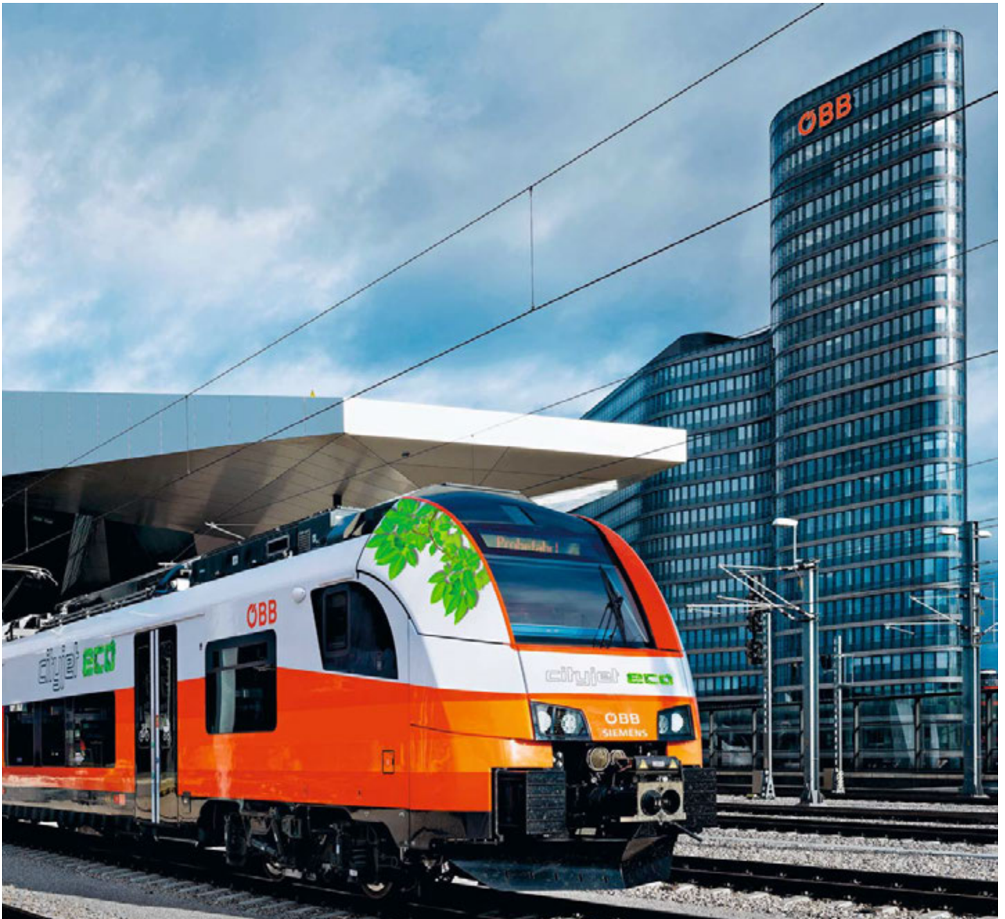
BATTERY OPERATED. The Cityjet eco will also travel using power on ancillary lines that have not been electrified
