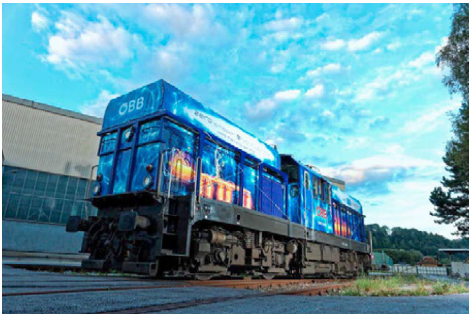
HYBRID SHUNTING LOCOMOTIVE. Intended for use in areas without overhead cables
