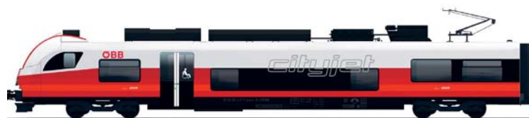
ÖBB-CITYJET. Length 75 m • Seats 244 (S-Bahn)/259 (regional train) • Weight 145 tonnes
